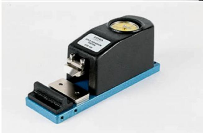
This well-proven instrument is designed to measure the strength of the adhesion of stuck-on and molded soles at the toe and heel of finished footwear in the shoe factory, but is equally useful in the testing laboratory.
