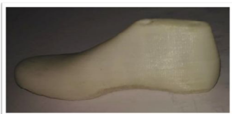
Fig.4 3D Printed Shoe last (Prototype)
